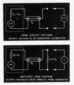
Figure 3. Output voltage calibration for a generator having its source impedance equal to the characteristic impedance of the output cable.
