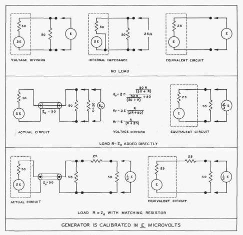
Figure 4. Application of Thevenin's Theorem to a cable terminated in Z<sub>o</sub>. TERMINATED CABLES ments with a signal generator has
