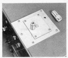
Figure 2. The Co-ax Adapter, mounted on an RX Meter. The 50-ohm termination shown beside the terminal plate is used in obtaining preliminary balance of the RX Meter bridge circuit.
