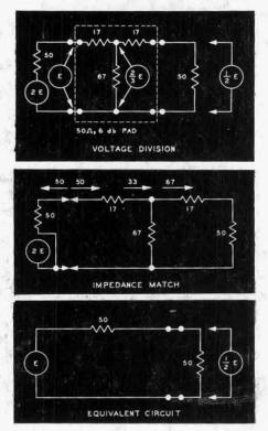
Figure 5. Equivalent circuit of a 50-ohm, 6 db symetrical attenuating pad. The output system should place at the end of a probe the equivalent antenna voltage and internal impedance.
