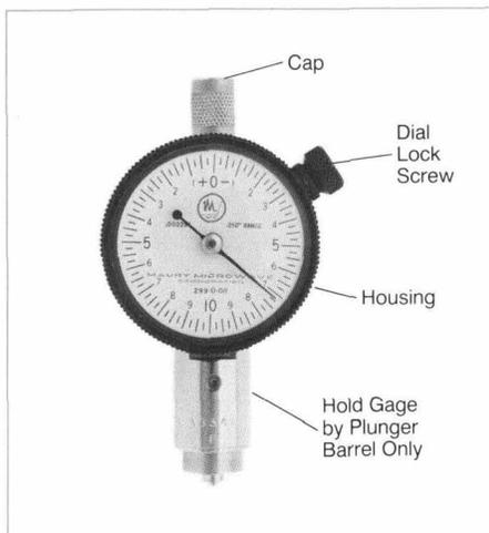
Figure 6. Using the Connector Gage
