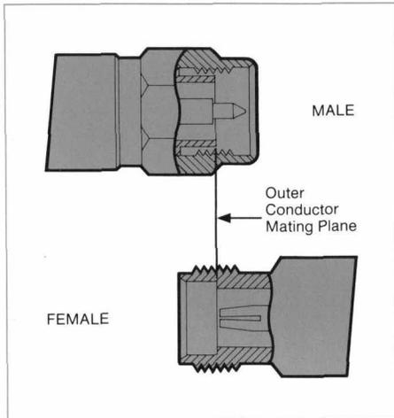
Figure 2. Precision 3.5mm connectors
