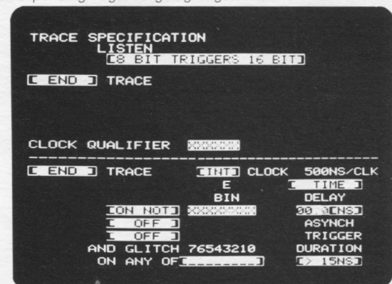
Figure 17. A "never trigger" trace specification (the logical not of "don't care") with [END] trace mode enables the 1615A to capture up to 256 bytes of data leading up to a system crash.
