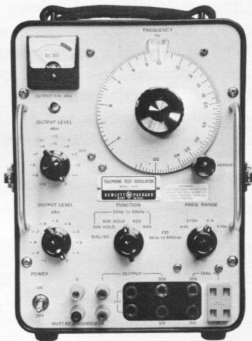
B. HP Model 236A 600 ohm 0 dBm Balanced Output Frequency = 1 kHz
